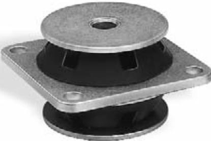
ET5220 Series All-Attitude isolators protect stationary loads of 15-50 lbs. and vehicular loads up to 30 lbs. from vibration, shock and noise.
