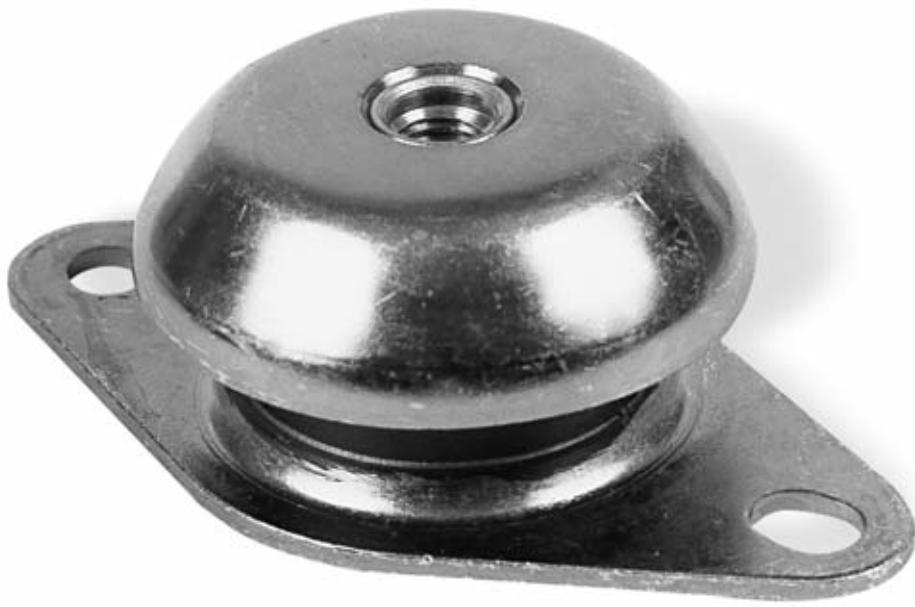
ITT Enidine Stable-Flex Mounts are specifically engineered to isolate lightweight, low-speed equipment. The complex geometry of the elastomer element in the mount provides a low-axial stiffness and excellent lateral stability.
