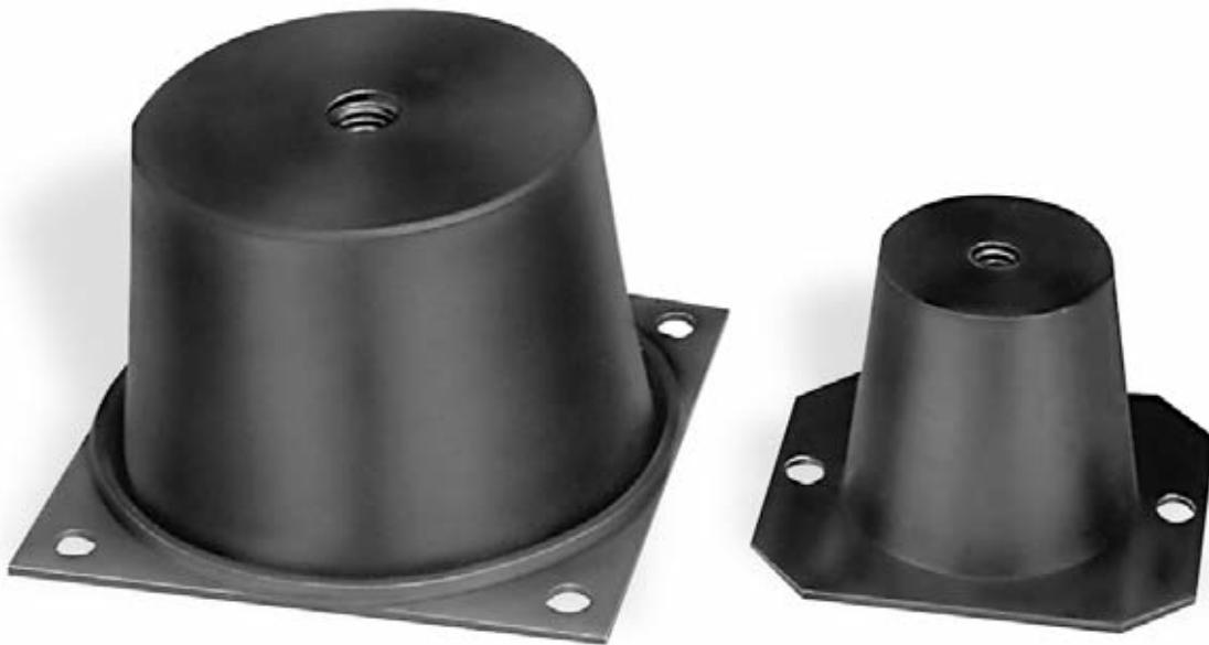
ITT Enidine Low Frequency Mounts have a unique design which bonds a steel spring inside a matrix of oil/ozone-resistant neoprene. The springs absorb low frequency vibrations, slowing and passing them onto the resilient neoprene. This material—made even more stable by the springs—interrupts the sound path, prevents noise amplification caused by sounding board effects and stops vibrations from being transmitted to the floor or work surface.
