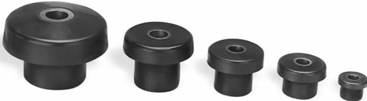
Here's the answer to fail-safe, multi-directional isolation in heavy-duty applications. During installation, a self-contained rebound is formed when a Center Bushing Mount's resilient element spreads under compression and the internal steel bushing serves as a positive spacer.
