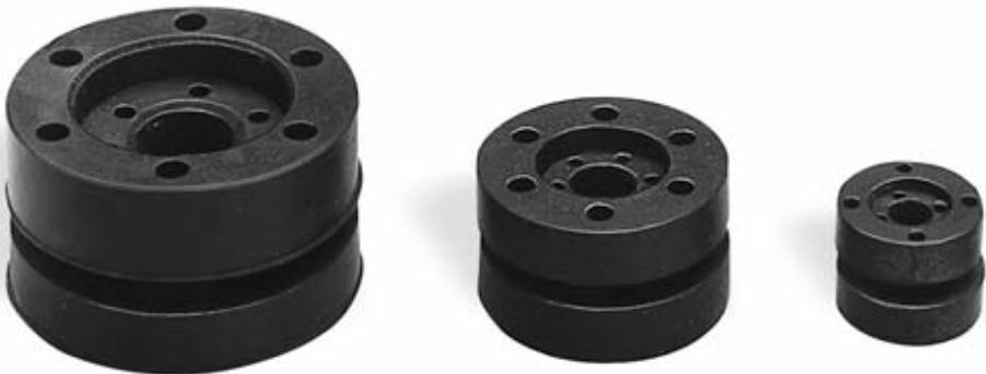
Neoprene Ring and Bushing Mounts are incorporated directly into the structural components of equipment such as office machines, motors and pumps, as well as air conditioning, electronic and scientific equipment. They offer fail-safe operation when installed in pairs.
