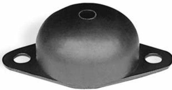
The interlocking metals of the Dome Mount series result in a fail-safe mount. This capability and low stiffness make them ideal for isolating medium to large sized engines as well as fans, blowers, pumps and air handling equipment.
