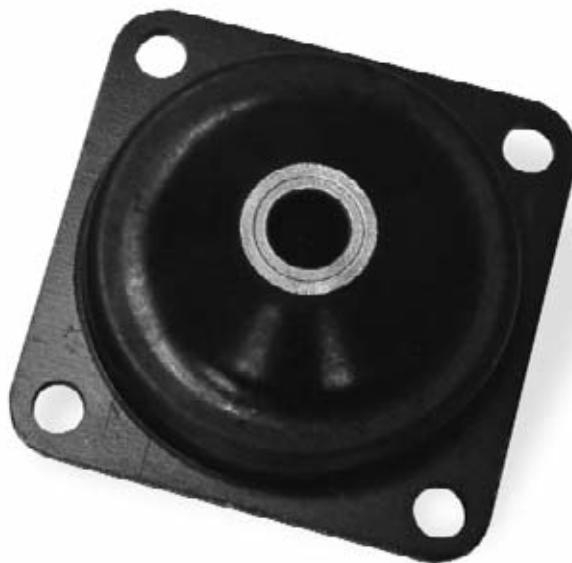
ITT Enidine Heavy Duty Plate Mounts provide excellent vibration isolation for applications where low natural frequency is required. At the rated loads, these mounts provide a natural frequency below 7 Hz. When used with snubbing washers, these mounts are fail-safe and can be used in very abusive applications.
