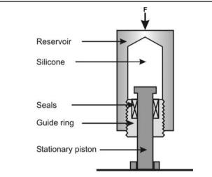
The load "F" forces the reservoir over the stationary piston. The silicone is compressed by the volume displacement of the stationarypiston.
