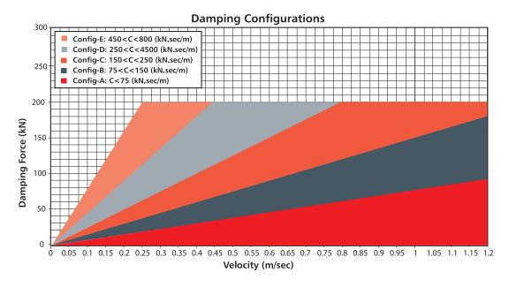
The FVD-B Series dampers are typically utilized on bridge and base isolation platforms requiring a long cycle life. This custom orifice designed damper provides the desired force versus velocity relationship symmetrically in both tension and compression directions, thermal compensation, and easy preventative maintenance inspection.
