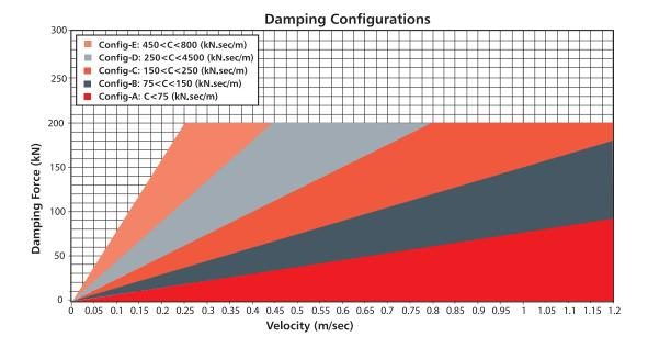
The FVD-B Series dampers are typically utilized on bridge and base isolation platforms requiring a long cycle life. This custom orifice designed damper provides the desired force versus velocity relationship symmetrically in both tension and compression directions, thermal compensation, and easy preventative maintenance inspection.
