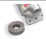
Wire mesh material can be manufactured in a multitude of shapes and sizes to accommodate your specific application. When exercised, the wire mesh damping elements convert input energy to heat. Friction is created when knitted or woven stainless steel wire strands are displaced relative to one another. Knitted metals have inherent resiliency and provide high-damping characteristics and non-linear spring rates.
