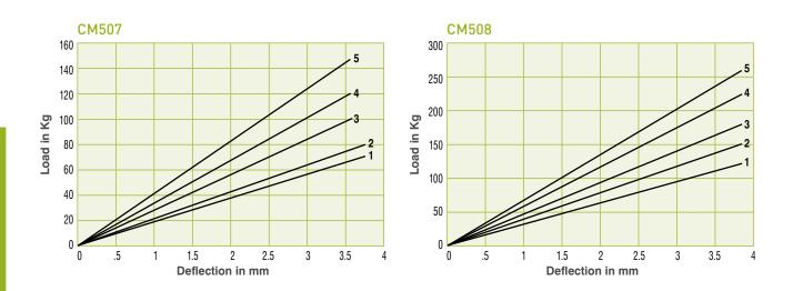
Max compression load in Kg deflection in mm.
