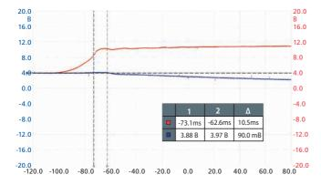
The magnitude of any pressure spikes exceeding the trip pressure which occur during deployment of the valve are dependant upon the system downstream volume: a larger system volume decreases the likelihood of the system pressure exceeding the trip pressure (see graphs). Any pressure spikes which do occur will only do so for a fraction of a second (less than the time taken for the device to operate).
